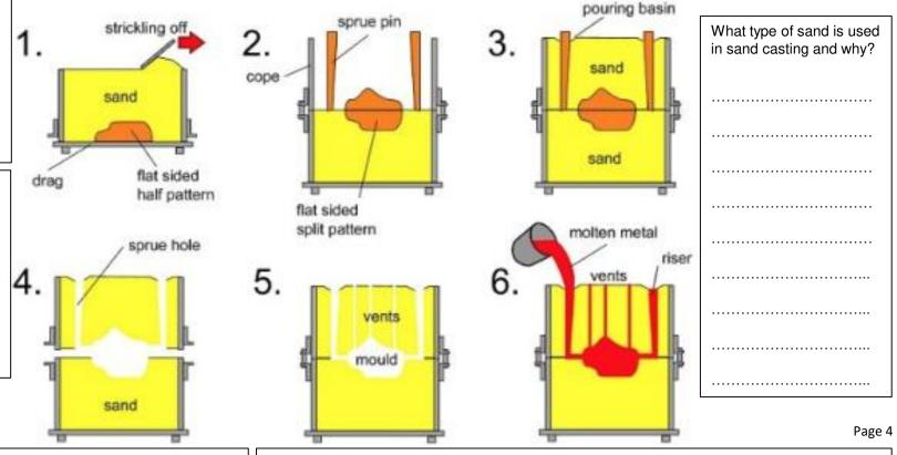
Stage 6: The extractor system must be turned on. The aluminium will be pre-melted and all of the correct PPE must be worn. The molten metal should be poured in a single smooth operation to prevent voids (air pockets) forming. The aluminium is then left to cool with the extraction hood placed over the top.
